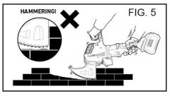
When using the Plunge blades, the cut should have enough clearance on each end (shown in Fig. 6), to ensure that no hammering of the blade ends occurs (as shown in Fig. 7).
